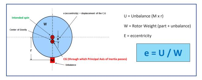
The above illustration shows a disk-shaped part, e.g., flywheel, gear, pump impeller, fan, etc. The mass **M**, at radius **r**, results in an unbalance **U**. Dividing the unbalance **U** by the weight **W** (rotor plus unbalance mass) gives us the eccentricity **e** (how far the rotor's mass center is displaced from the
