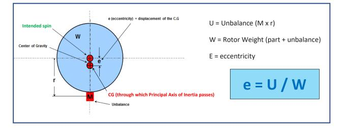
The above illustration shows a disk-shaped part, e.g., flywheel, gear, pump impeller, fan, etc. The mass **M**, at radius **r**, results in an unbalance **U**. Dividing the unbalance **U** by the weight **W** (rotor plus unbalance mass) gives us the eccentricity **e** (how far the rotor's mass center is displaced from the intended spin axis).
